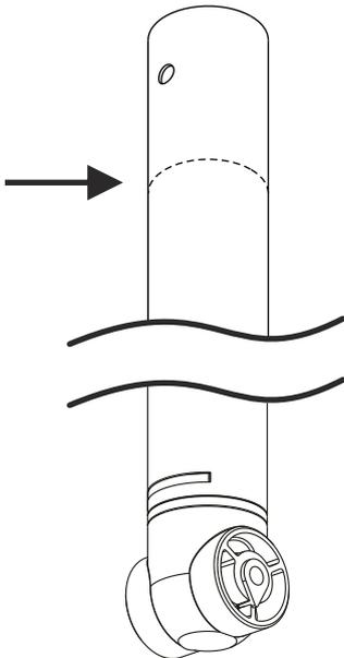
**b** Re-drill 9mm hole through approx 30mm from pole top
