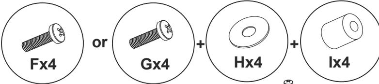
**Note:** Use the appropriately sized fixings from the fixing kit. Use spacers as required, not always necessary.
